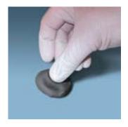
2. Mix by kneading with gloved fingers to a uniform color. If mixing is difficult, warm AM 103 Rapid Cure Metal Stick to room temperature or slightly above.
